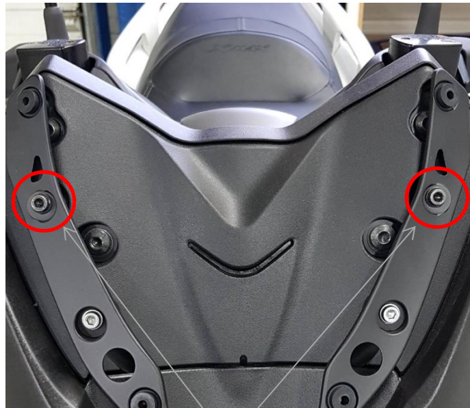
Location of the screws to replace
